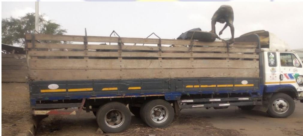
Figure 8: Livestock transport truck with wooden side walls and vent, but without roof
