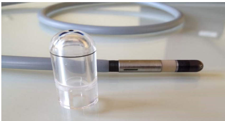
Figure 16: 0.125 cc Semiflex ionisation chamber and its build-up cap
