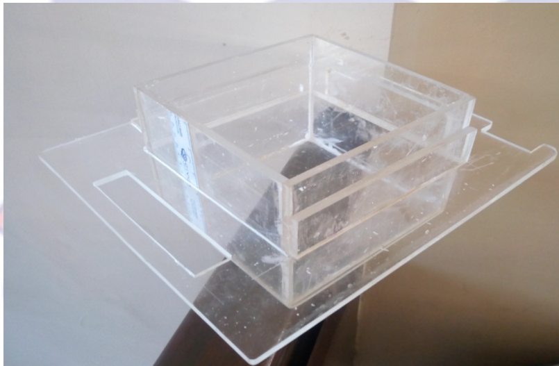
Figure 27: Locally fabricated tanks that can be mounted on the collimator system of Equinox 100 cobalt 60 teletherapy machine
