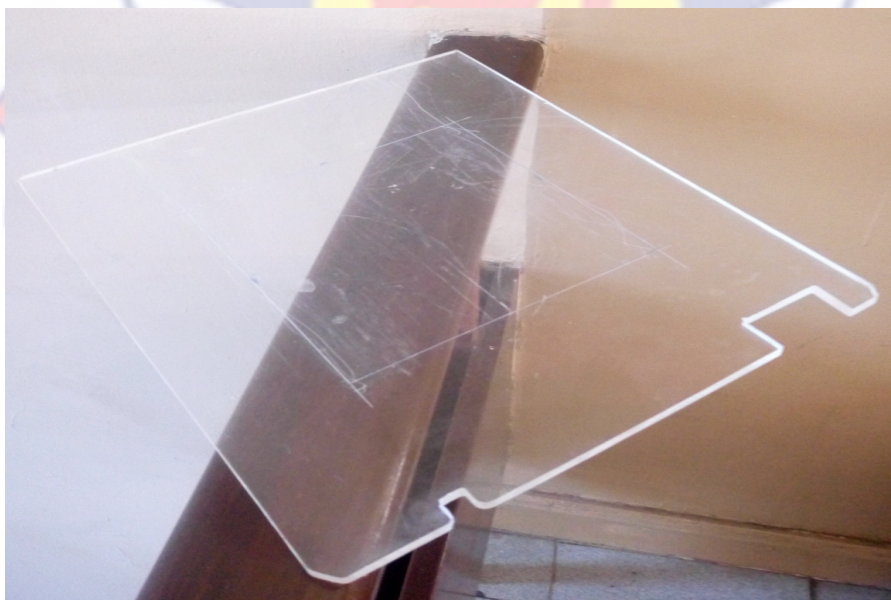
Figure 28: Sample of block tray in use by the oncology department for mounting customized shielding blocks
