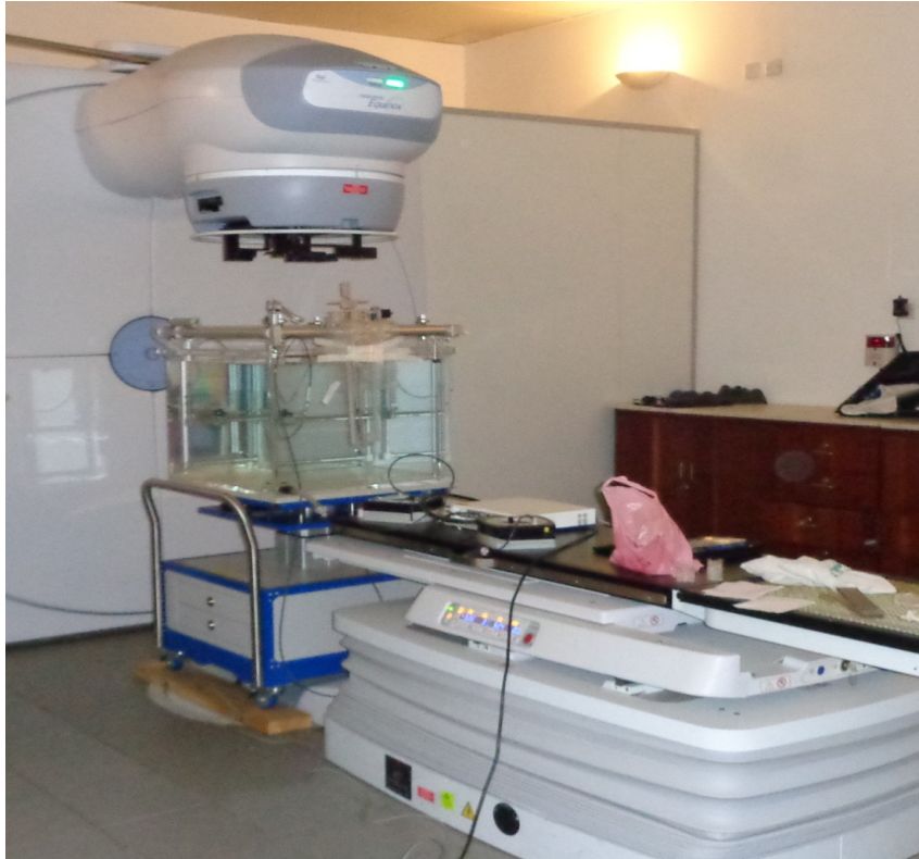
Figure 31: Equinox 100 telecobalt machine and Blue phantom 2 motorised water tank set-up for beam data acquisition
