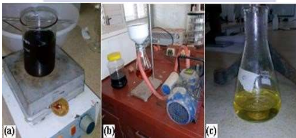
Figure 9: Sample preparation: (a) - activated charcoal mixed with the RBPKO (b) - the vacuum filtration process that separated the activated charcoal from the oil (c) the final 'bleached' RBPKO.
