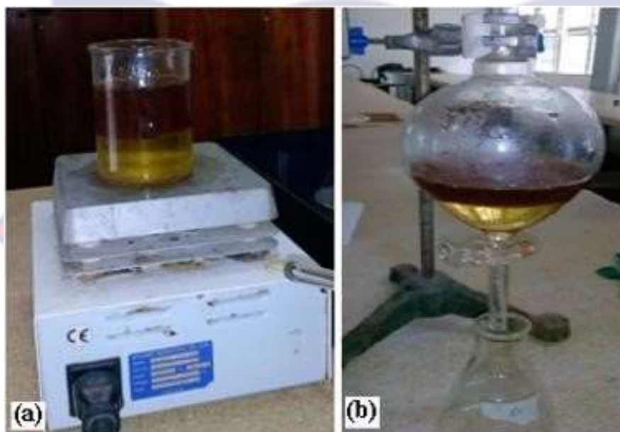
Figure 7: Sample Preparation (A) – the crude PKO and Distilled Water being heated on a Hot-Plate. (B)– The mixture being separated using a Separating Funnel
