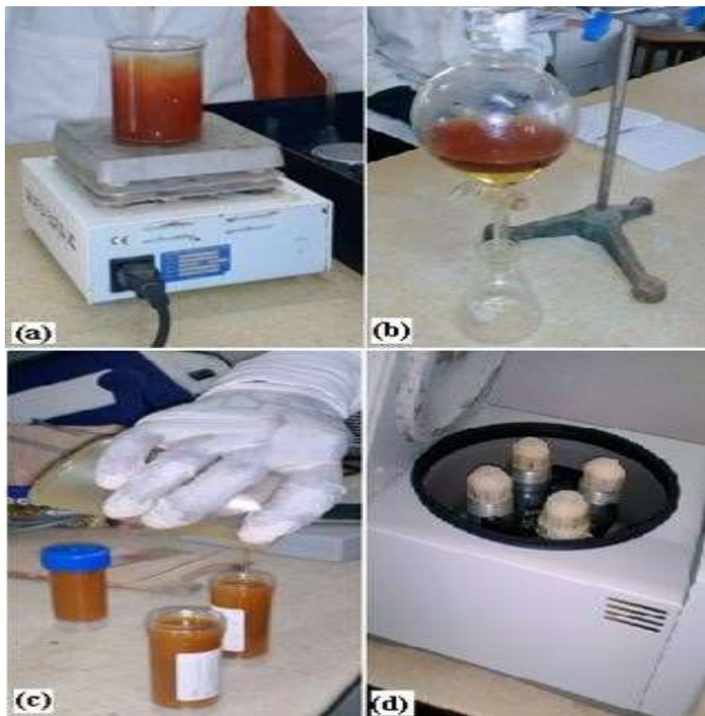
Figure 8: (a) Sample preparation, (b) Oil treatment with Phosphoric acid. (c) Treatment with Sodium Hydroxide and (d) the mixture centrifuged
