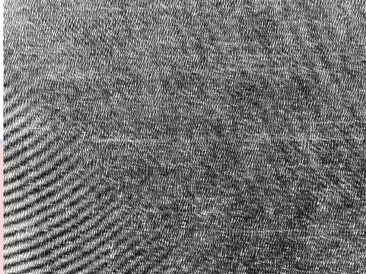
Figure G: The off-axis reflection configuration of the recorded interferogram of the marble plate.
