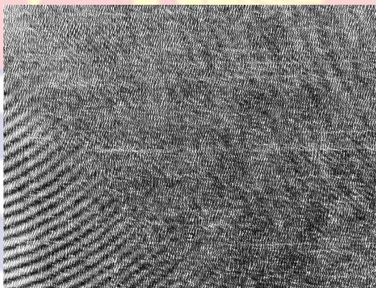
Figure 19a: The interferogram recorded of the letters ‘ROU’
