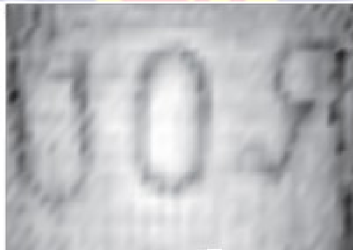
Figure 20b: Amplitude reconstruction of the letters 'ROU' after zero padding operation
