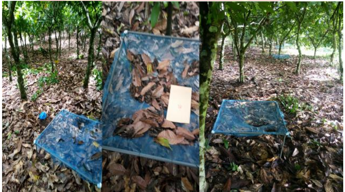
Figure 2: Litter traps installed to collect litter at two-monthly intervals for the period.
