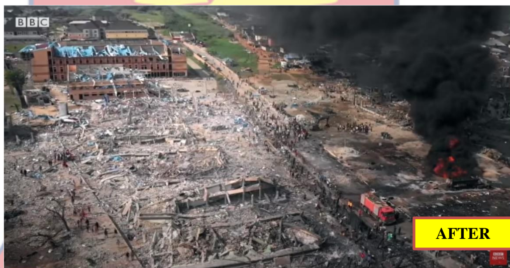
Plate 5: After effects of a vapour cloud explosion in Lagos, Nigeria. 16th March, 2020.
