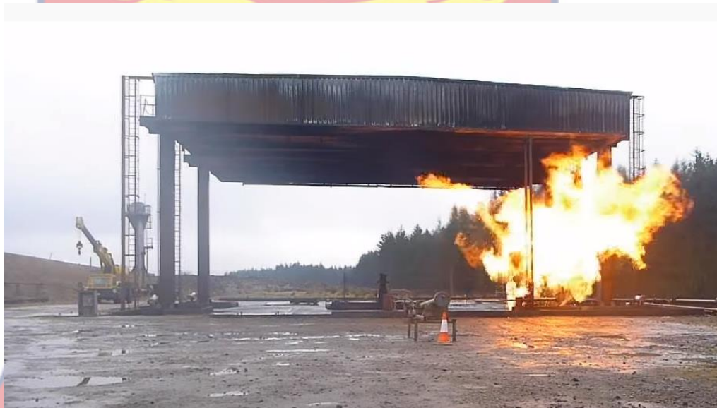
Plate 3: Flash fire at a test site Source: Process Engineering Channel, YouTube, 2015.
