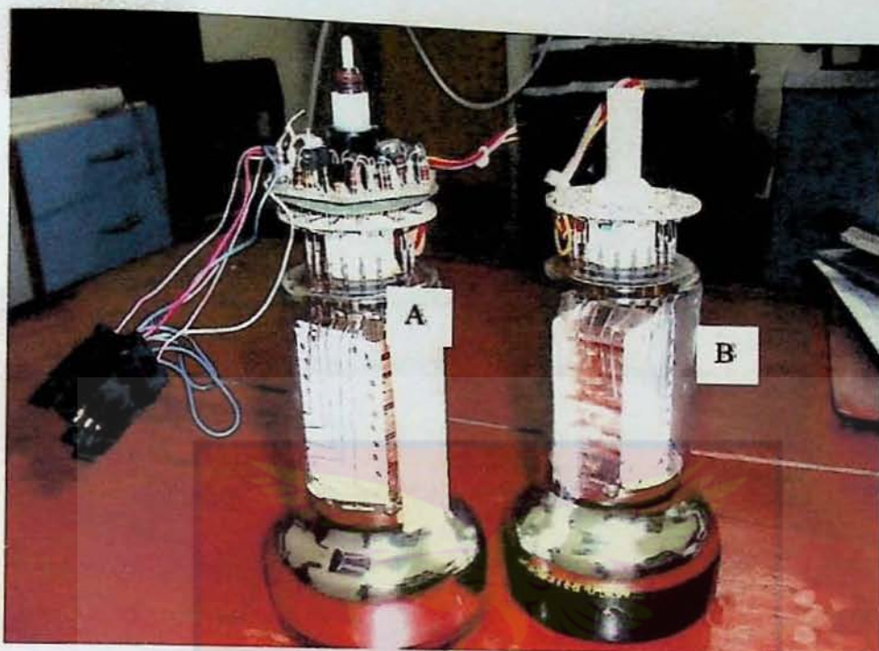
Plate 14: Two of the PMTs that were tested under this work A) With preamplifier was used for the PMT with preamp measurement. B) PMT with no preamp connected was used PMT without preamp measurement.
