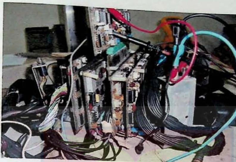
Plate 16: Analyzer 1, board is placed on a PCB extender board and is being aligned for zero offset voltages
