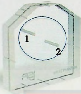
Figure 17: Wilke phantom with defined length dimension
