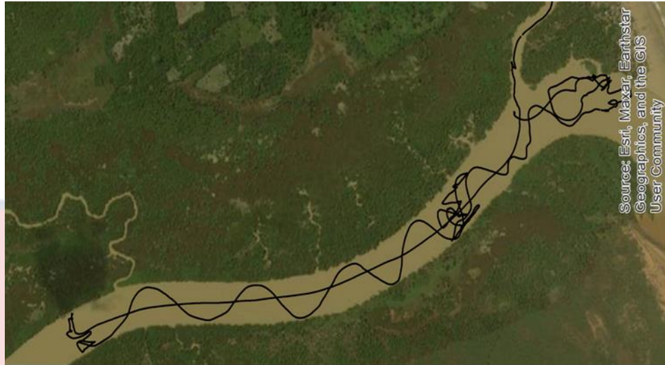
Figure 3.5: Depth measurement across the Pra Estuary
