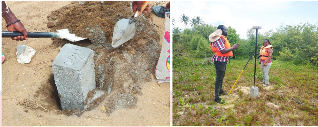
Figure 3.6: GCPs establishment at Anlo Beach
