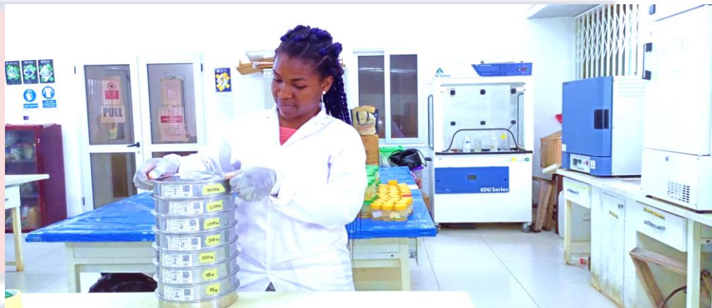
Figure 3.11: Sieving of sediment samples for particle size analysis
