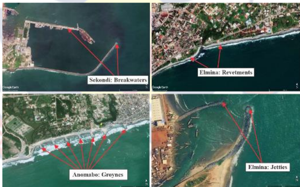
Figure 2.10: Examples of sea defence structures used on the coast of Ghana and towns in which they are located. Source: Google Earth Pro (2022)
