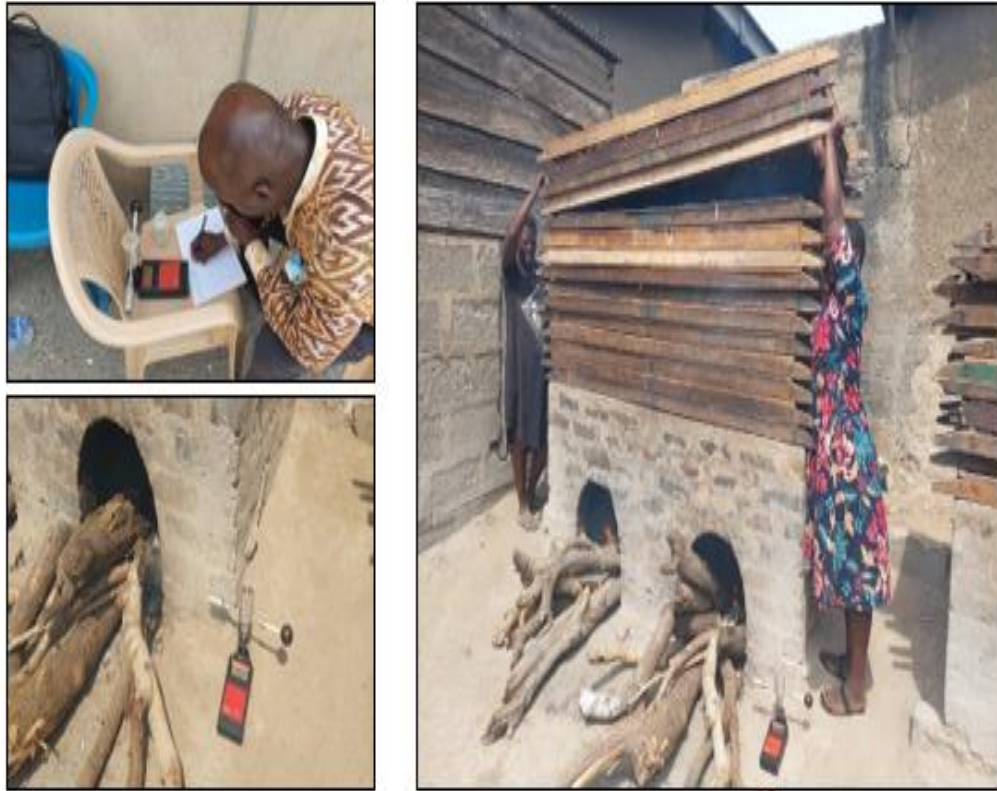
Plate 1: Measuring a Fish Smoker's Heat Stress Monitoring Using HSM 100 CASELLA Monitor (Casella CEL. (2022)).
