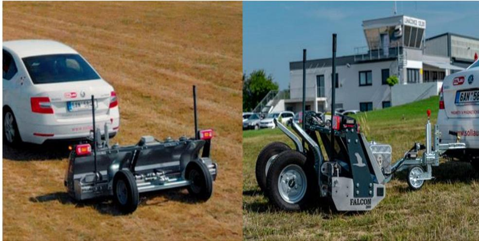
Figure 5: Picture of the FALCON MS magnetic sweepers (ACCGAC, n.d.)
