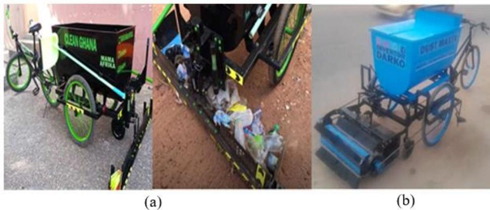
Figure 2: Pictures of some sweeper tricycles with mechanical brooms
