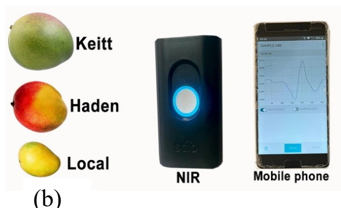
Figure 2.15: (a) NIRQuest spectrometer (Raghavendra et al., 2021) (b) SCIO NIR spectrometer with the three varieties of mango fruits (Lamptey, Teye, Abano, & Amuah, 2023) (Published under open access)
