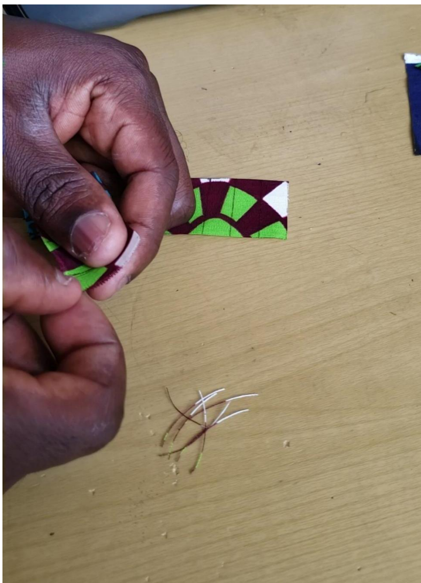
Picking ends for yarn count
