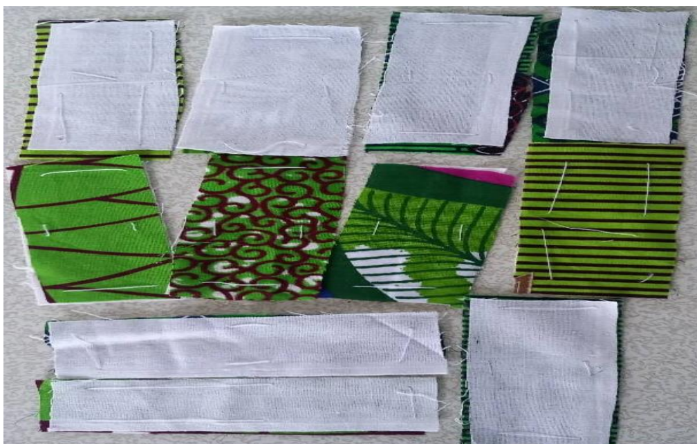
Figure 10: Printed and white fabrics stitched together for colourfast test
