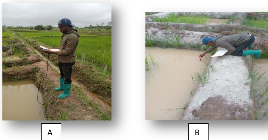
Figure 6: Determination of water quality (A) Use of oxyguard to record dissolved oxygen and temperature (B) Use of electronic pH meter to record water pH.
