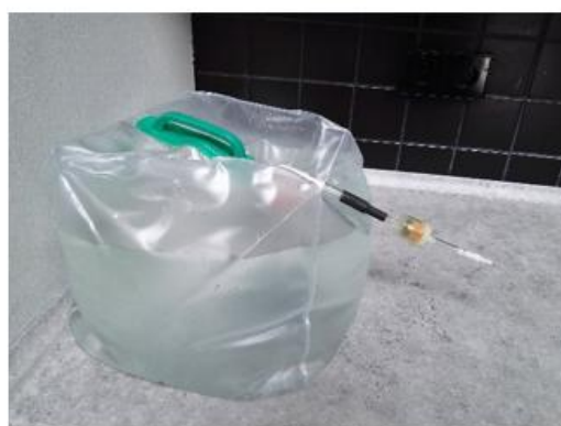
Water tank, with valve, water filter and hose-connector to irrigation line.
