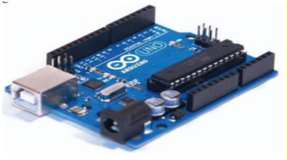
Figure 45: Arduino Uno microcontroller board (Badamasi, 2014)
