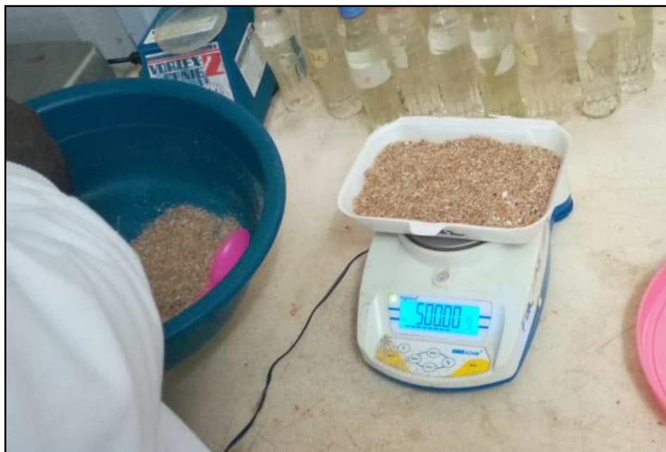
Plate 2: Electronic weighing scale used for assessing 500 g of sampled sediment Source: Department of Fisheries and Aquatic Science's laboratory, UCC (2021).
