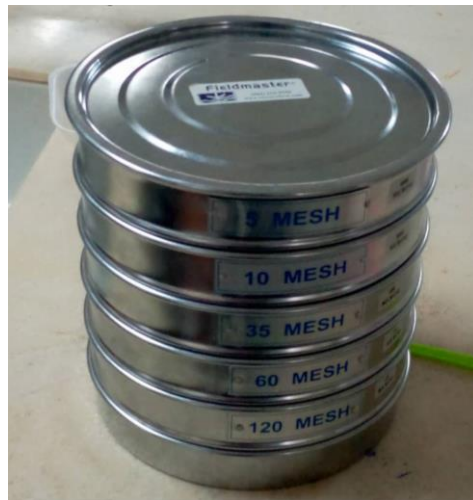
Plate 1: Fieldmaster's Dry Sieve set used at the laboratory for the particle size analysis.
