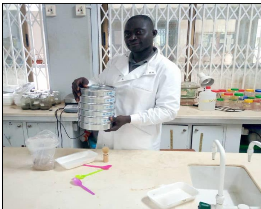
Plate 3: Manual shaking of sieves set by the researcher Source: Department of Fisheries and Aquatic Science's laboratory, UCC (2021).
