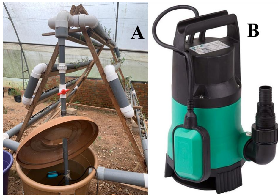
Figure 3.5: Image of storage tank and hydroponic system – A and submersible pump (Rio SPW 1100) – B.
