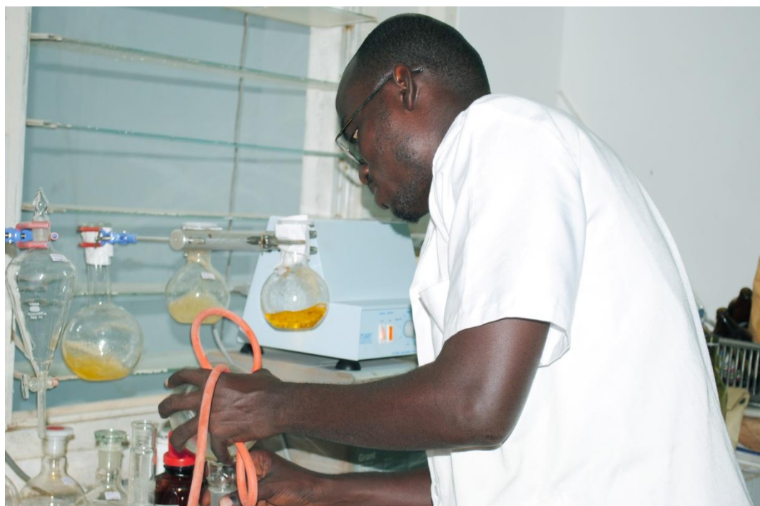
Figure 1: A laboratory picture showing pesticide extraction using a flask shaker
