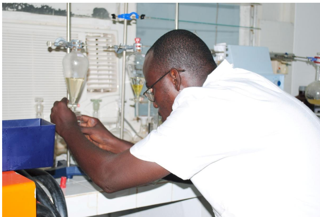
Figure 2: A laboratory picture showing separation of extract after partition
