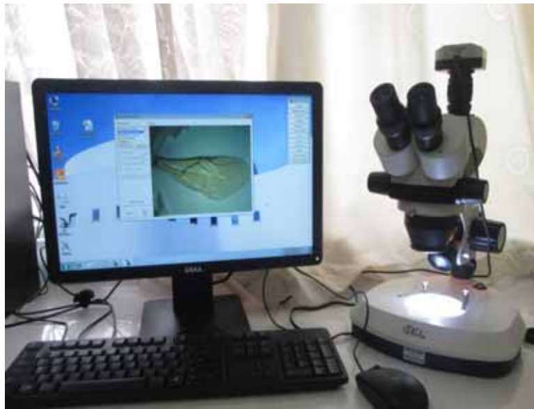
Plate 14: Set up for image acquisition using the stereomicroscope
