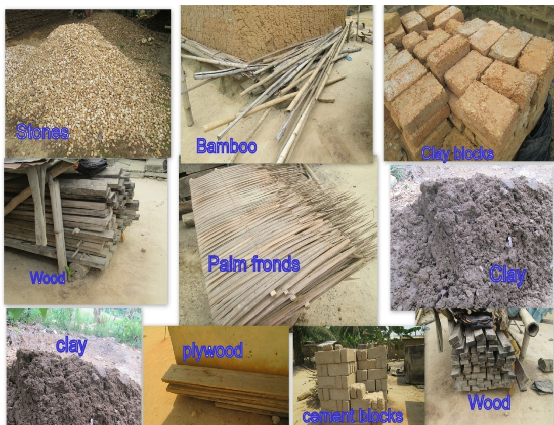
Plate 2: Some materials used to construct the household latrines
