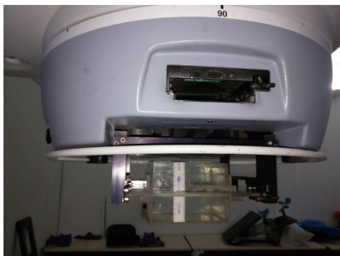
Figure 2. Locally fabricated water tank mounted on the accessories holder of telecobalt machine during measurement of attenuation coefficient of water.
