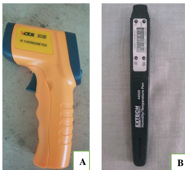
Figure 15: Infra-Red Thermometer Victor 303B (A) and the RH-44550 Pen (B) used to measure temperature and relative humidity.
