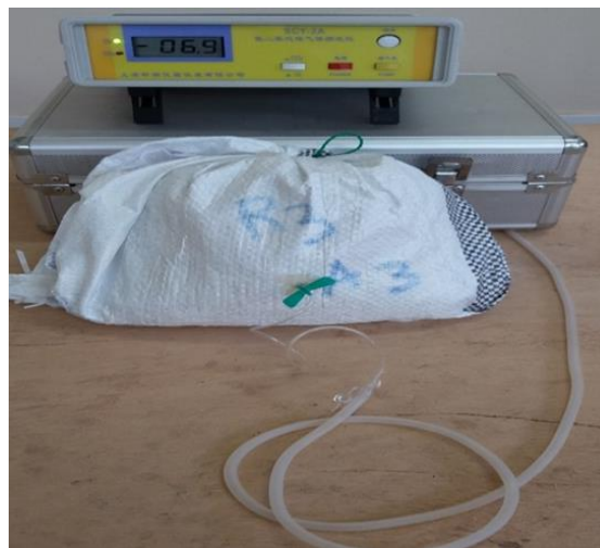
Figure 16: Recording oxygen concentration using GrainPro oxygen Analyzer.
