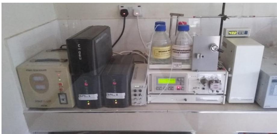
Figure 18: A Cecil Adept Binary Pump High Pressure Line Chromatograph (HPLC) for aflatoxin analysis.
