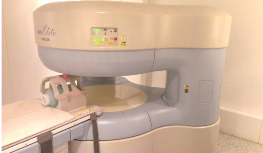
A 0.3 T Permanent Magnet Airis Elite Machine Used at the Diagnostic Centre Limited Manufactured by Hitachi Medical Corporation.
