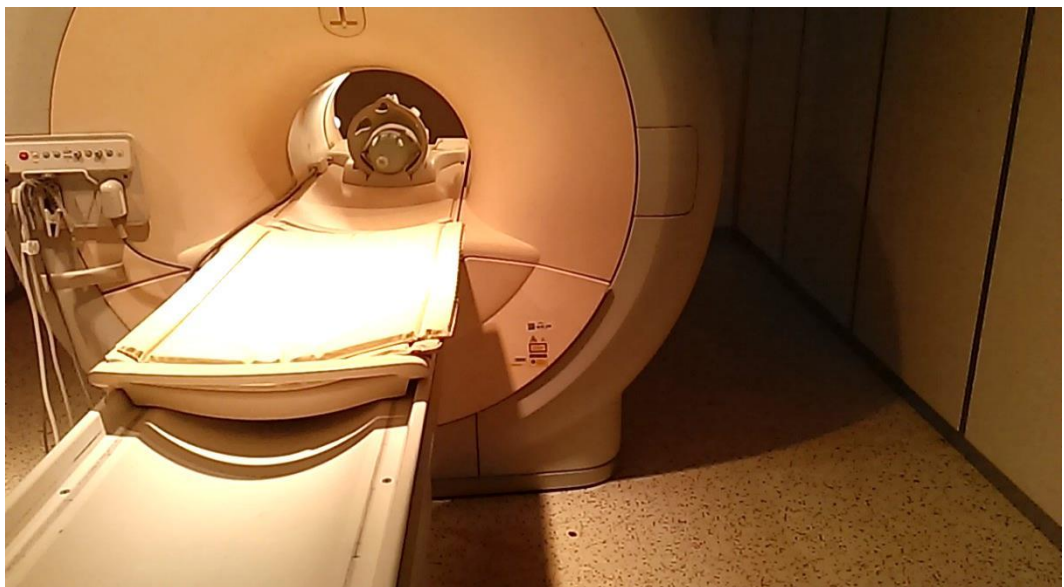
A 1.5 T Superconducting Magnet MR Machine Used at the 37 Military Hospital Manufactured by Philips.
