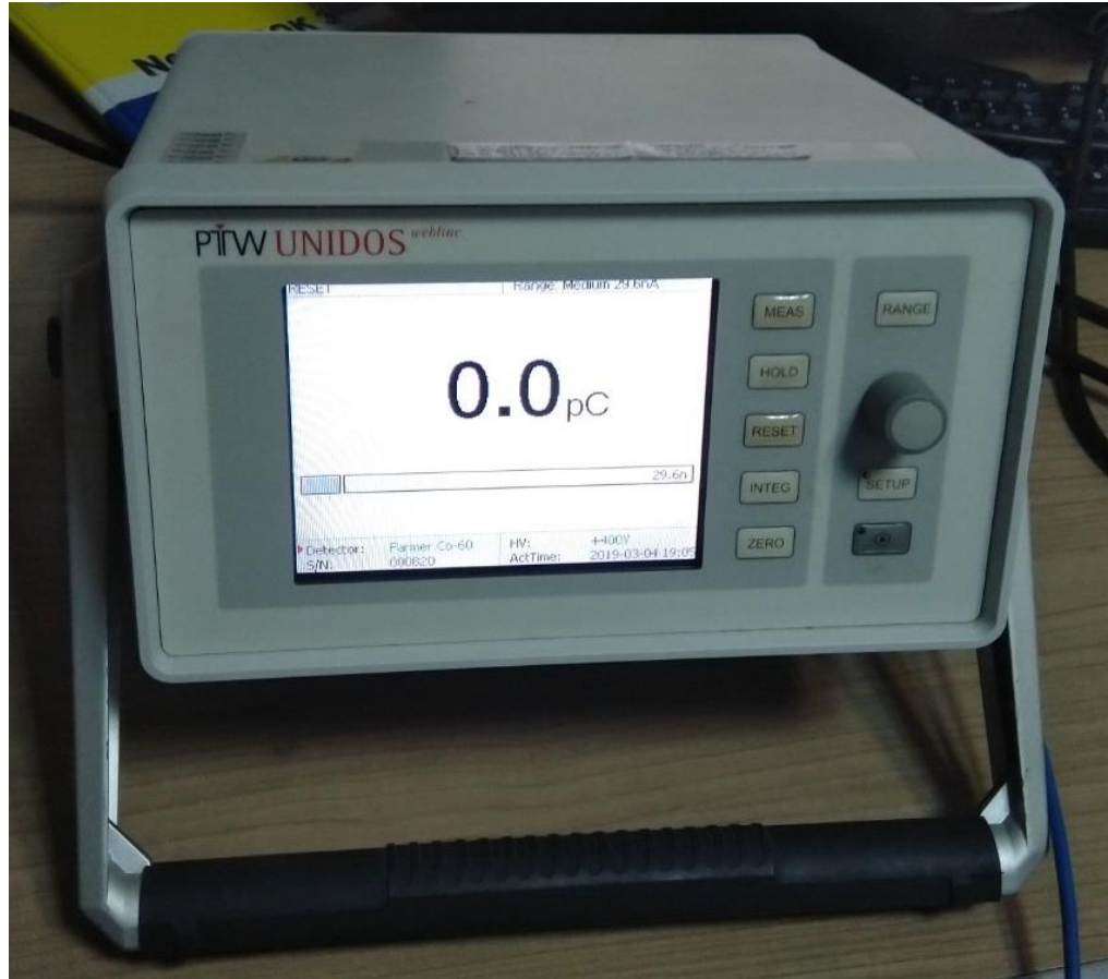
Figure 12: PTW-UNIDOS Electrometer used in this study for reference measurements of dose in the PMMA solid water phantom (Field
