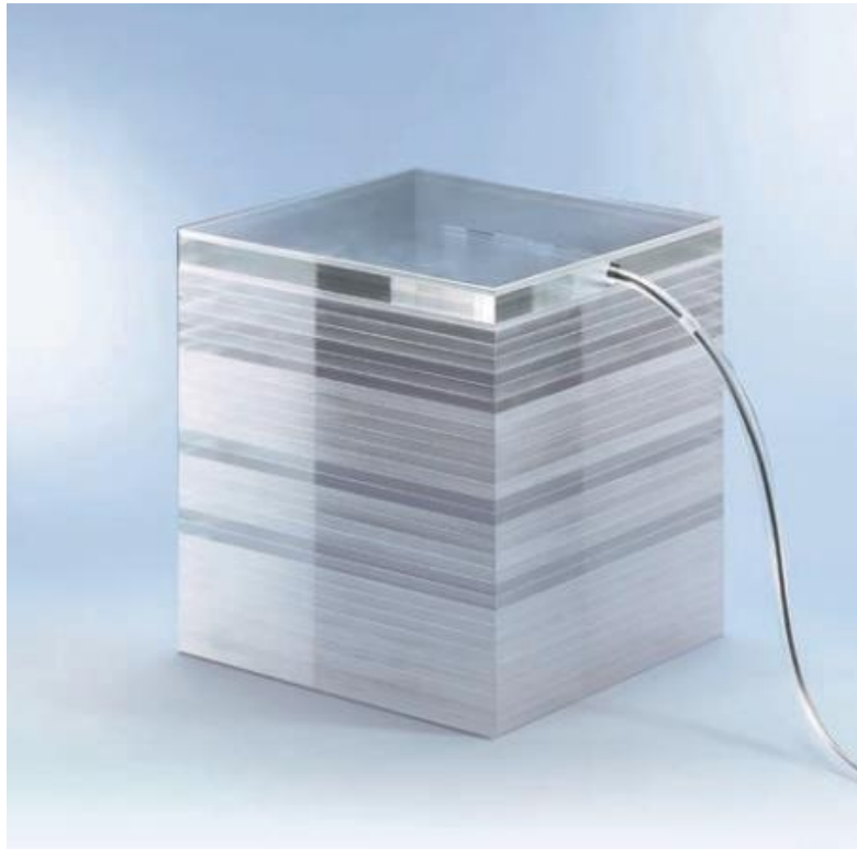
Figure 2: PMMA slab phantoms used for absolute dosimetry (Ion Beam Applications (IBA), 2013)
