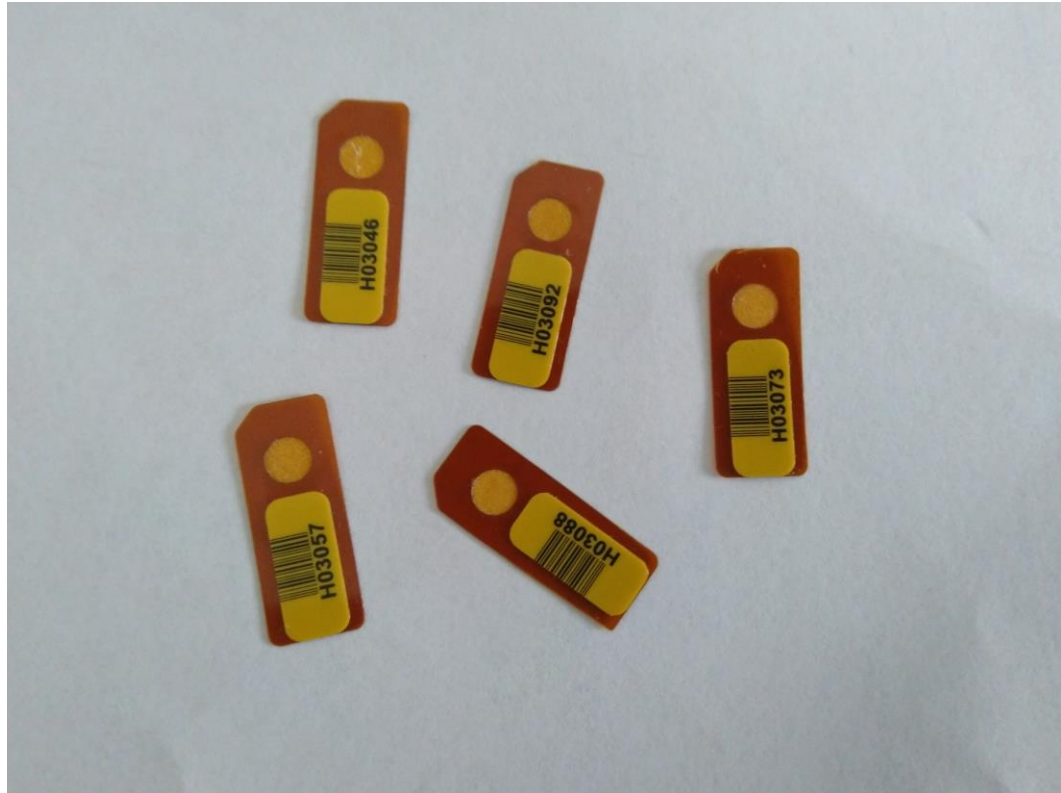
Figure 13: LiF:Mg, Ti TLDs used for transit dosimetry model evaluation (Field Work, 2018)
