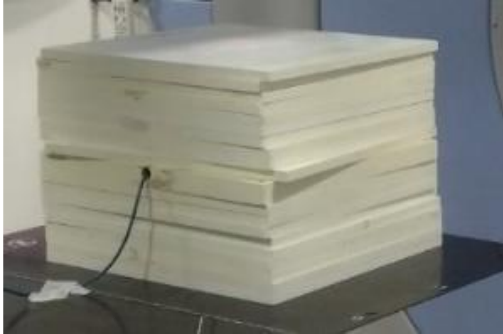
Figure 16: 30 cm × 30 cm PMMA phantom slabs (manufactured by PTW) used in this study. Each slab has a thickness of 1 cm (Field Work, 2017)
