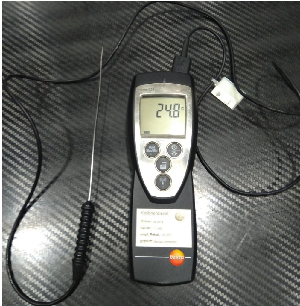
Figure 14: Testo 925 Thermometer used in this study (Field Work, 2017)
