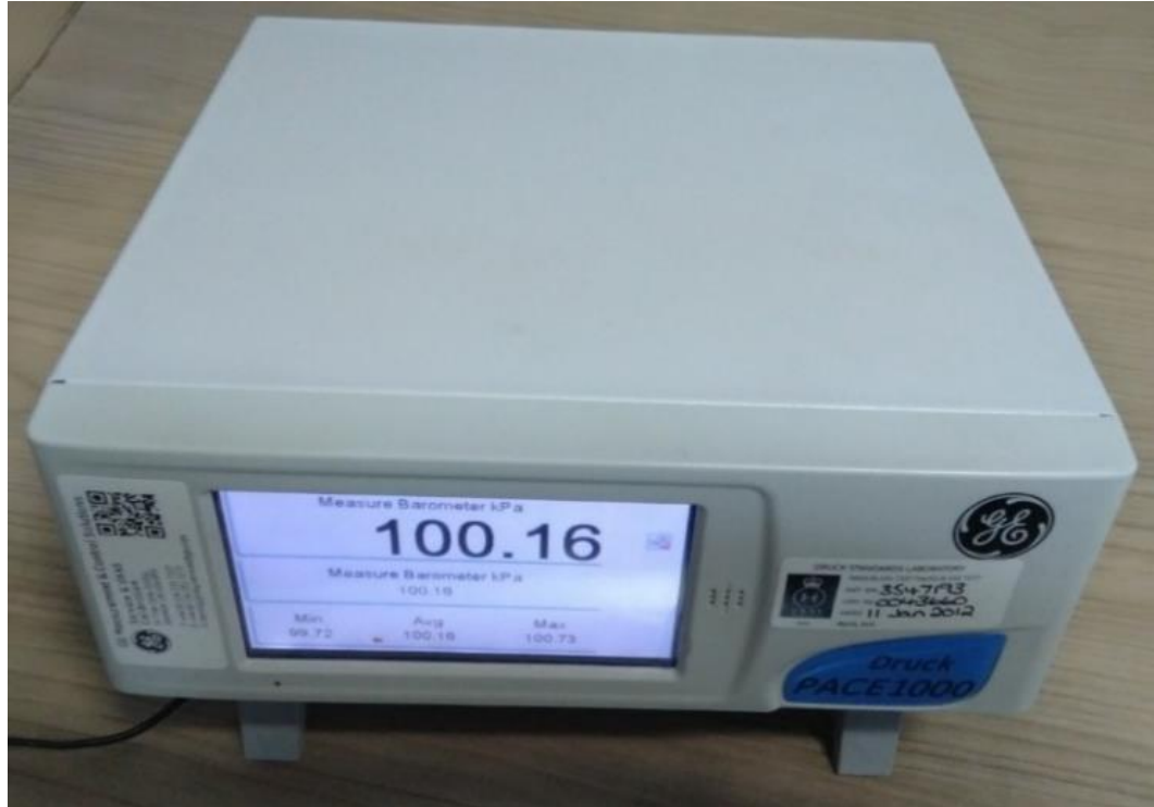
Figure 15: GE Druck Barometer PACE 1000 used in this study (Field Work, 2017)
