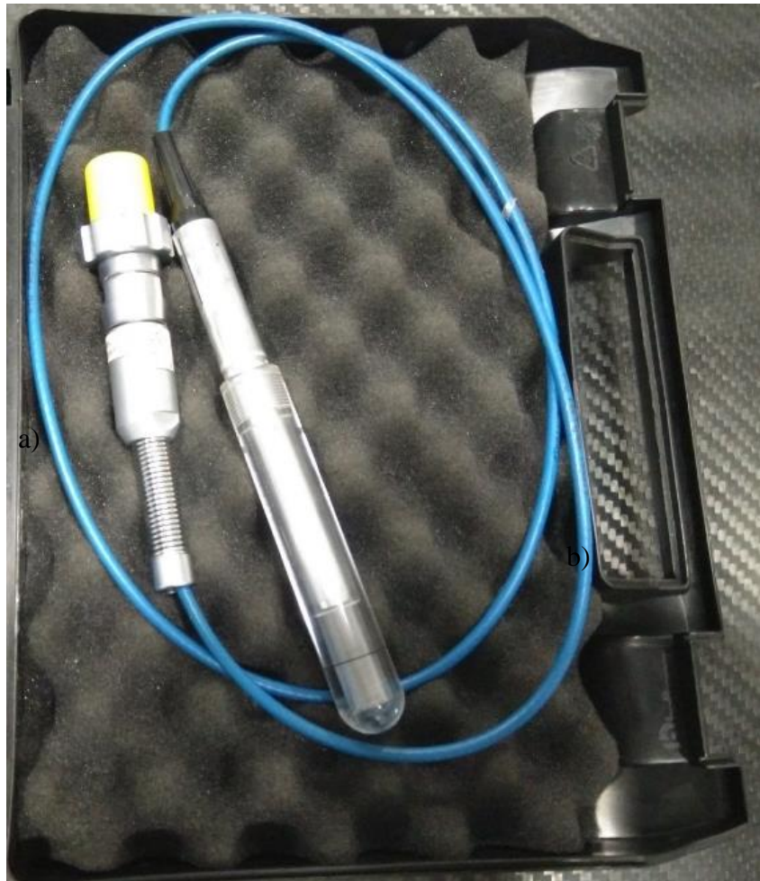
Figure 11: Farmer-Type PTW IC 30010 used in this study for reference measurements of dose in the PMMA solid water phantom (Field Work, 2017)
