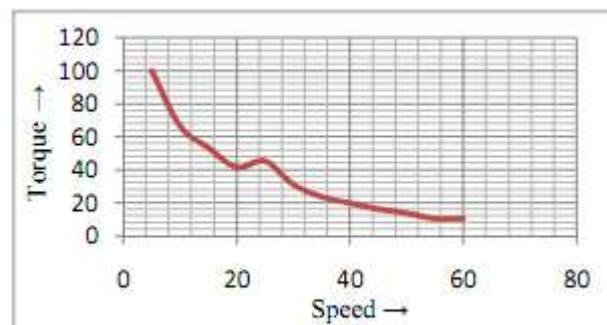
Figure 5. Graph of speed torque characteristics of dc motors
