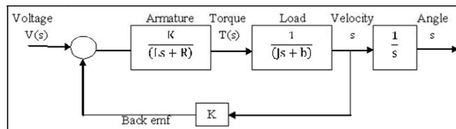
Figure 4. Block diagram of DC motor
