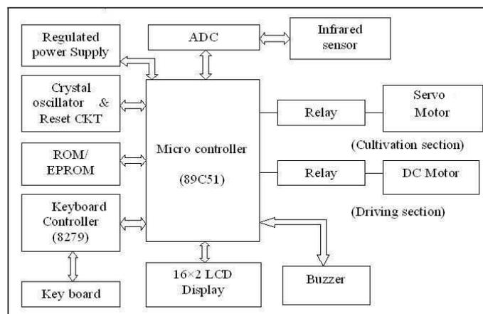
Figure 1. Hardware structure of Robotic system.
