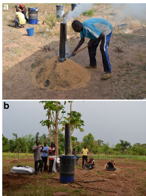
Fig. 1 Carbonization of rice husks by farmers in the field using the Japan retort (a) and the ELSA barrel (b)
