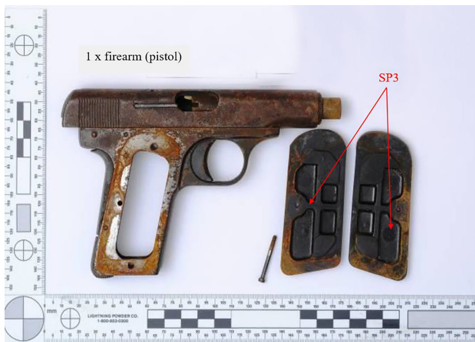
Fig. 1. A disassembled pistol with the inside of the hand grip shown. The red arrows (SP3) indicate the inside surface of the hand grip (a protected area), which was swabbed. The firearm was discarded in a stormwater drain and recovered nine days later following a period of torrential rain. A good DNA profile was obtained after swabbing under the grip (plastic), while other parts of the firearm swabbed yielded no profile. (Picture Courtesy: Dr Jennifer Raymond, Research Coordinator, Forensic and Technical Services Command, NSW Police Force, Australia. Image used with permission). (For interpretation of the references to colour in this figure legend, the reader is referred to the web version of this article.)
