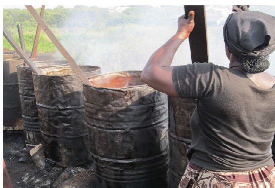
Oil producing reactors with a worker stirring the heating mixture
