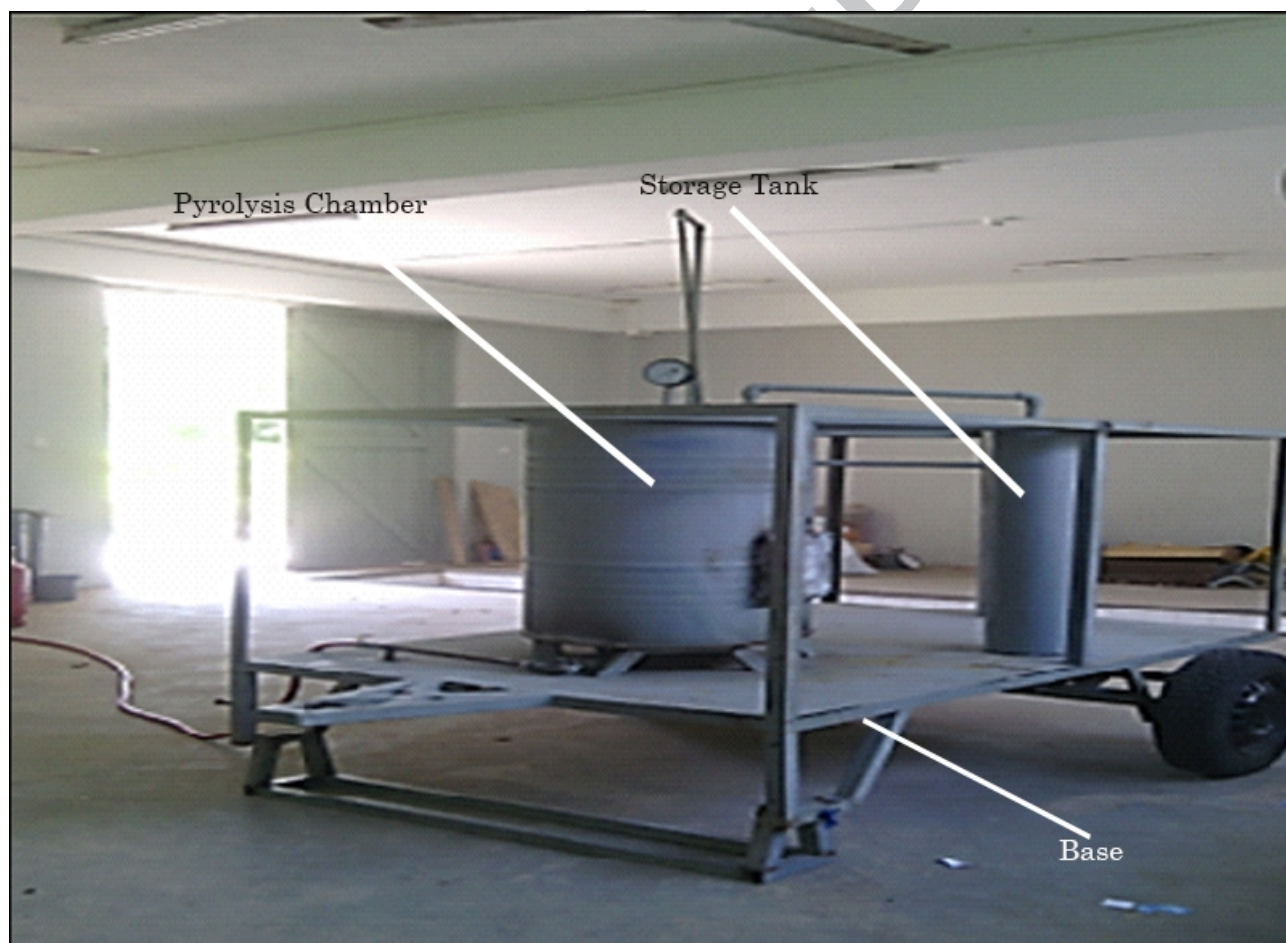
Fig. 2 - A Diagrammatic presentation of the pyrolysis process picture of the pyrolysis movable setup.
