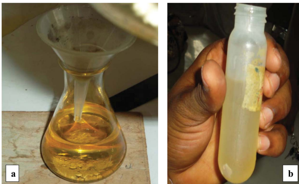
Figure 3. (a) Crude glucoamylase after filtration. (b) Supernatant of centrifuged glucoamylase.
