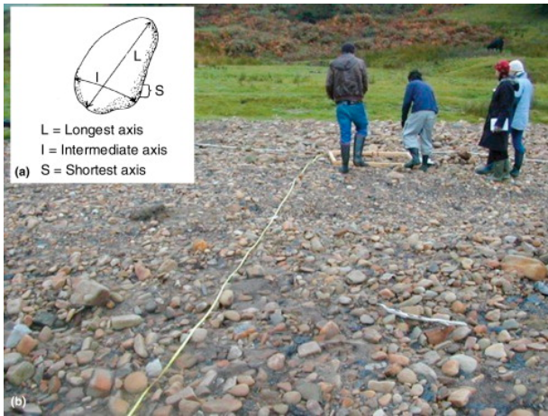
Figure 3. (a) The measuring approach to pebbles for a Wolman pebble count. (b) Students conduct Wolman pebble counts in the Ashop River, Derby County, England. Photograph courtesy of Farah Alamgir, Loughborough University.
