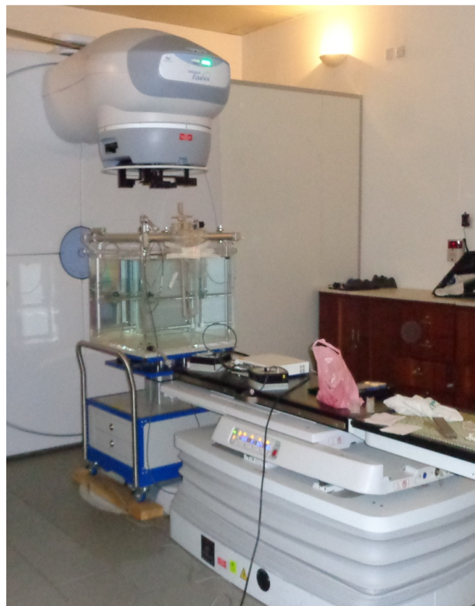
Figure 1. Telecobalt machine with beam measuring equipment (Blue Phantom 2 water phantom) in the path of beam.
