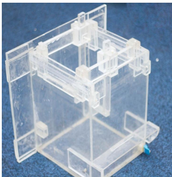
Figure 2: Cross sectional view of the locally constructed water phantom
