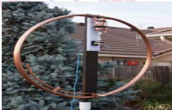
Figure 15: A photograph of a large loop antenna
