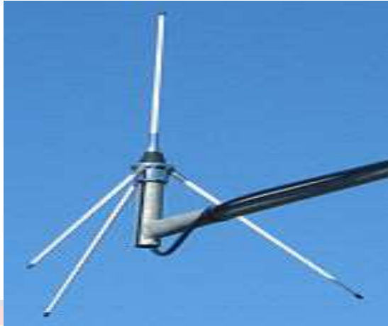
Figure 6: A photograph of a Monopole antenna
