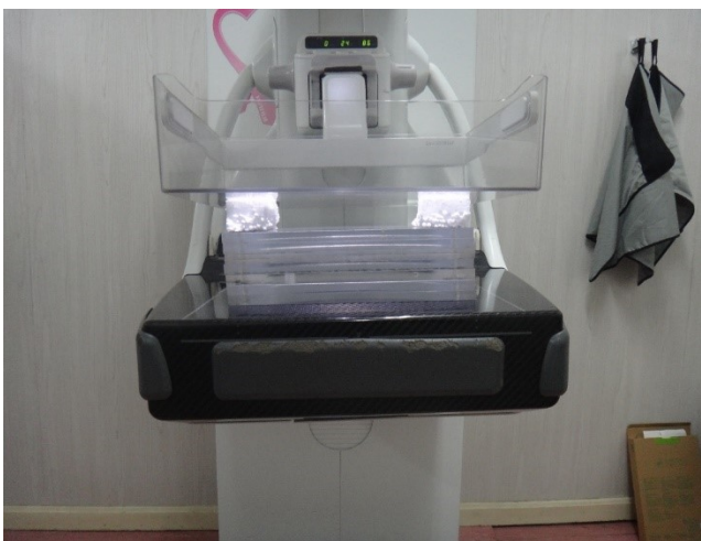
Figure 3: Set – up for Image quality test on 70 mm phantom with spacer to obtain an equivalent breast thickness of 90 mm
