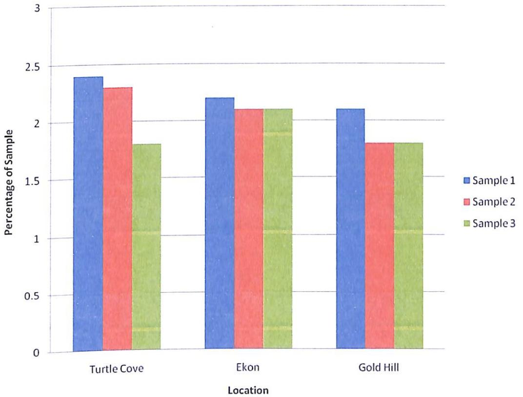
**Figure 13: Percentage of clay in the near shore. Source: Field data (2013).**
