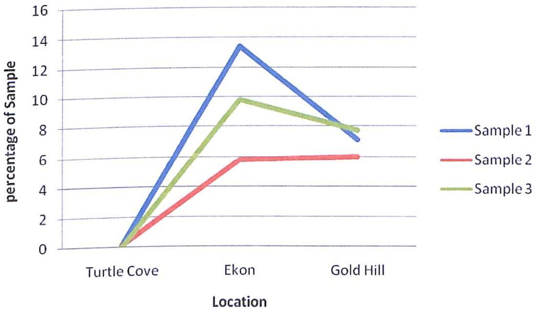
**Figure 9: Percentage of fine sand in the near shore. Source: Field data (2013).**
