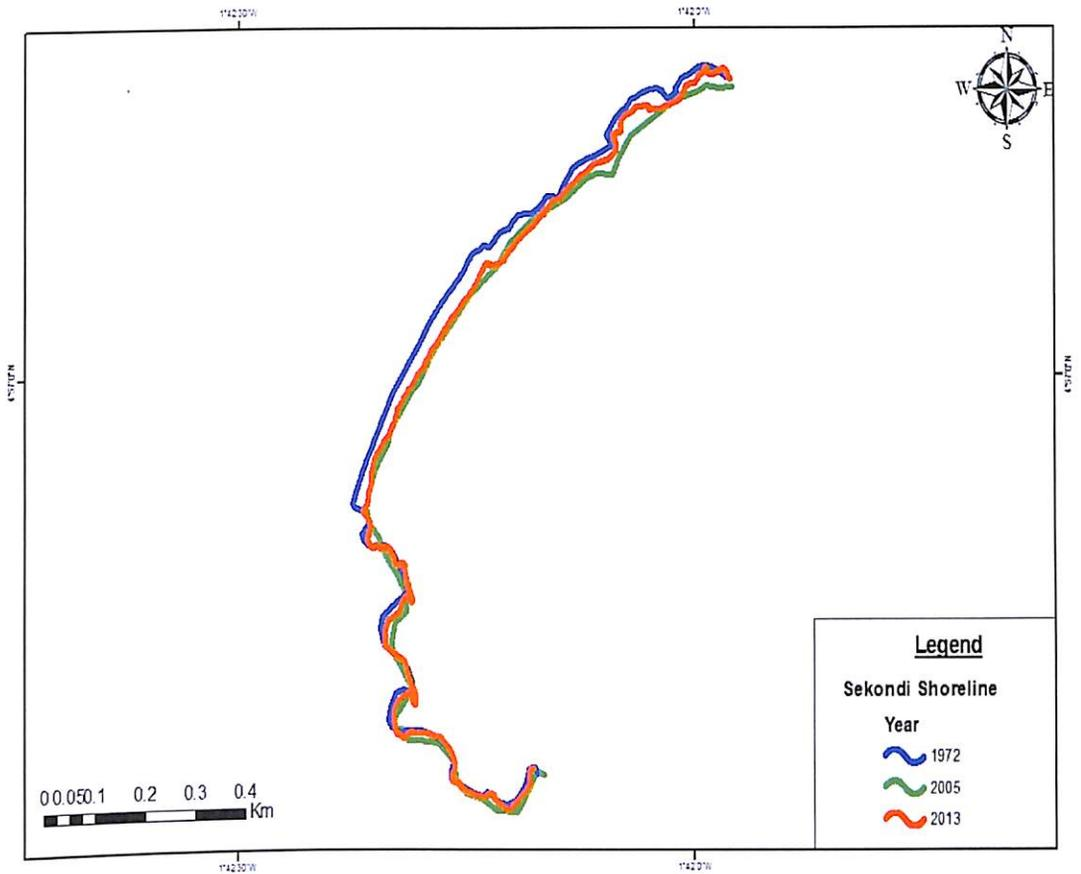
**Figure 21: Shoreline positions of Sekondi for 1972, 2005 and 2013**
