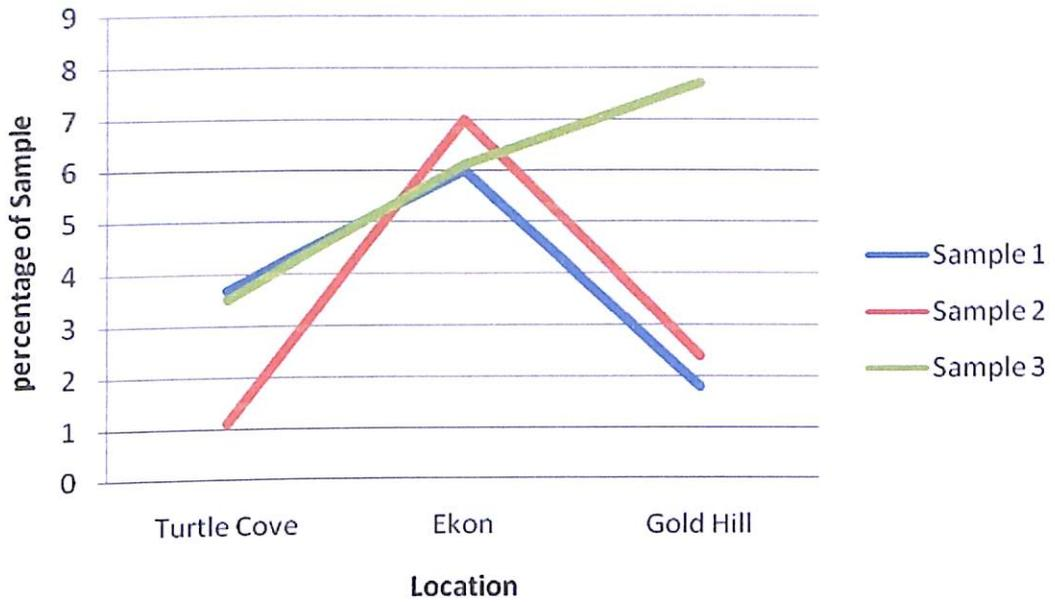
**Figure 10: Percentage of fine sand in the upper reaches. Source: Field data (2013).**
