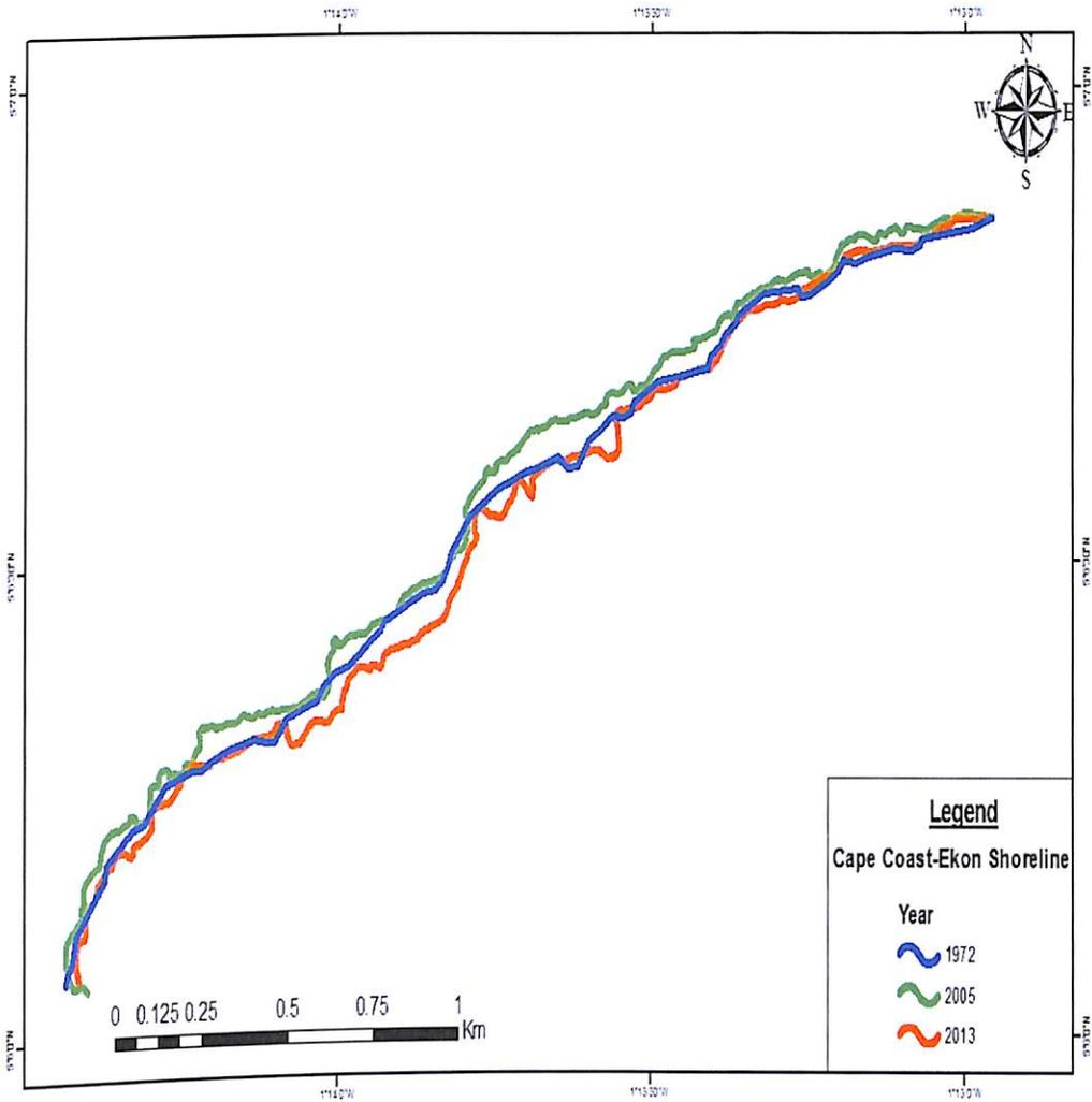
**Figure 15: Shoreline positions in Ekon and Cape Coast for 1972, 2005 and 2013. Source: Field survey (2014).**
