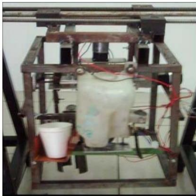
(a) The structure of the transplanter
