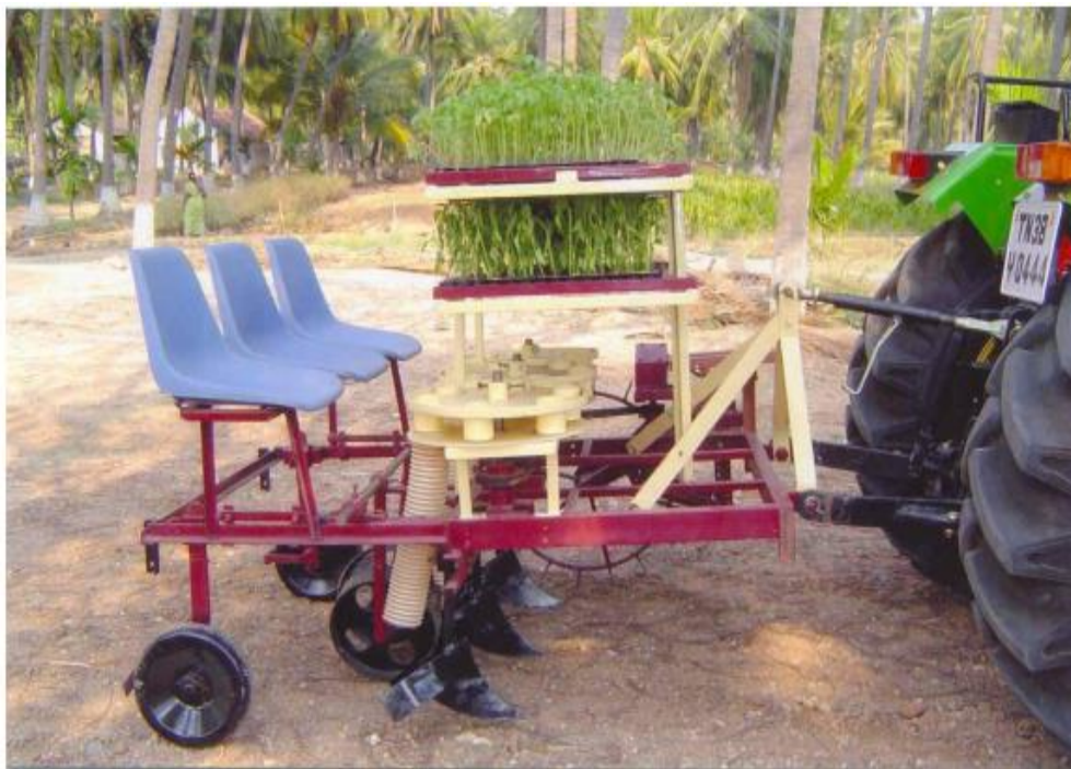
Figure 5: Tractor operated three row plug type vegetable transplanter (Kavitha and Karunanithi, 2008)
