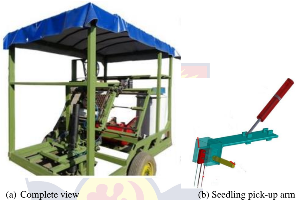
Figure 13: The fully automatic single-row vegetable transplanter (Zamani, 2014)
