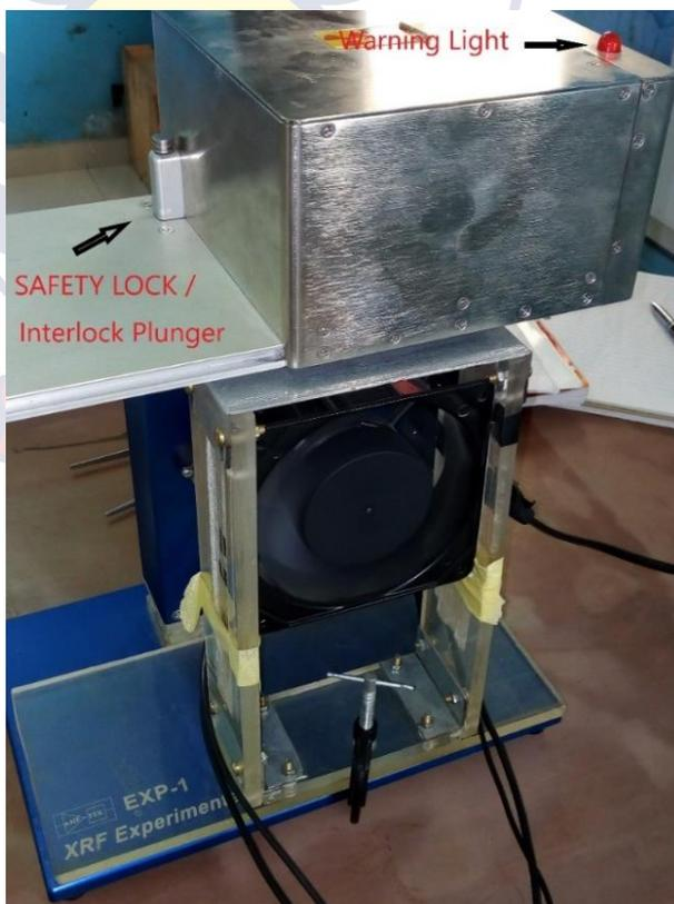
*Figure 13:* The shielding compartment with safety plunger showing the safety features of the AMPTEK EXP 1 X-123 XRF experimenter kit.
