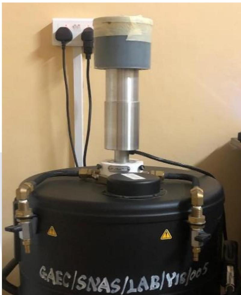
*Figure 17: Detector-Beaker configuration*
