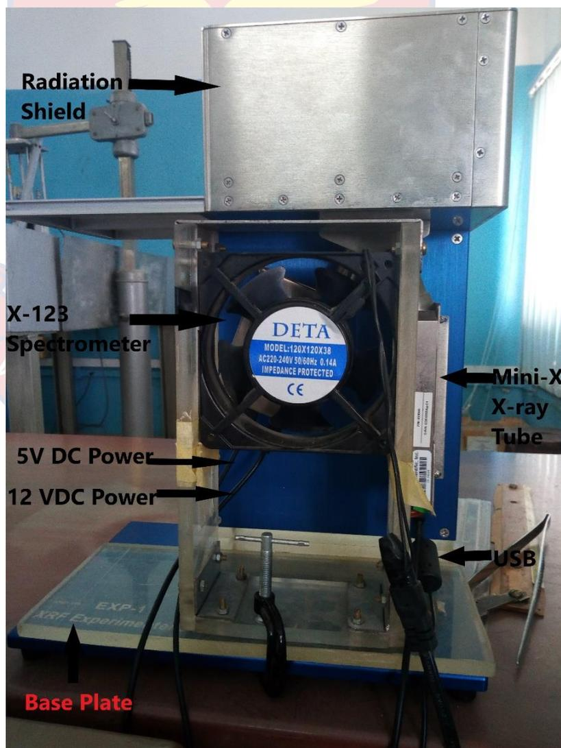
Figure 12: AMPTEK EXP-1 X-123 XRF experimenter kit showing the radiation source (Mini-X-ray Tube) and spectrometer (X-123) both situated beneath the radiation shielding compartment
