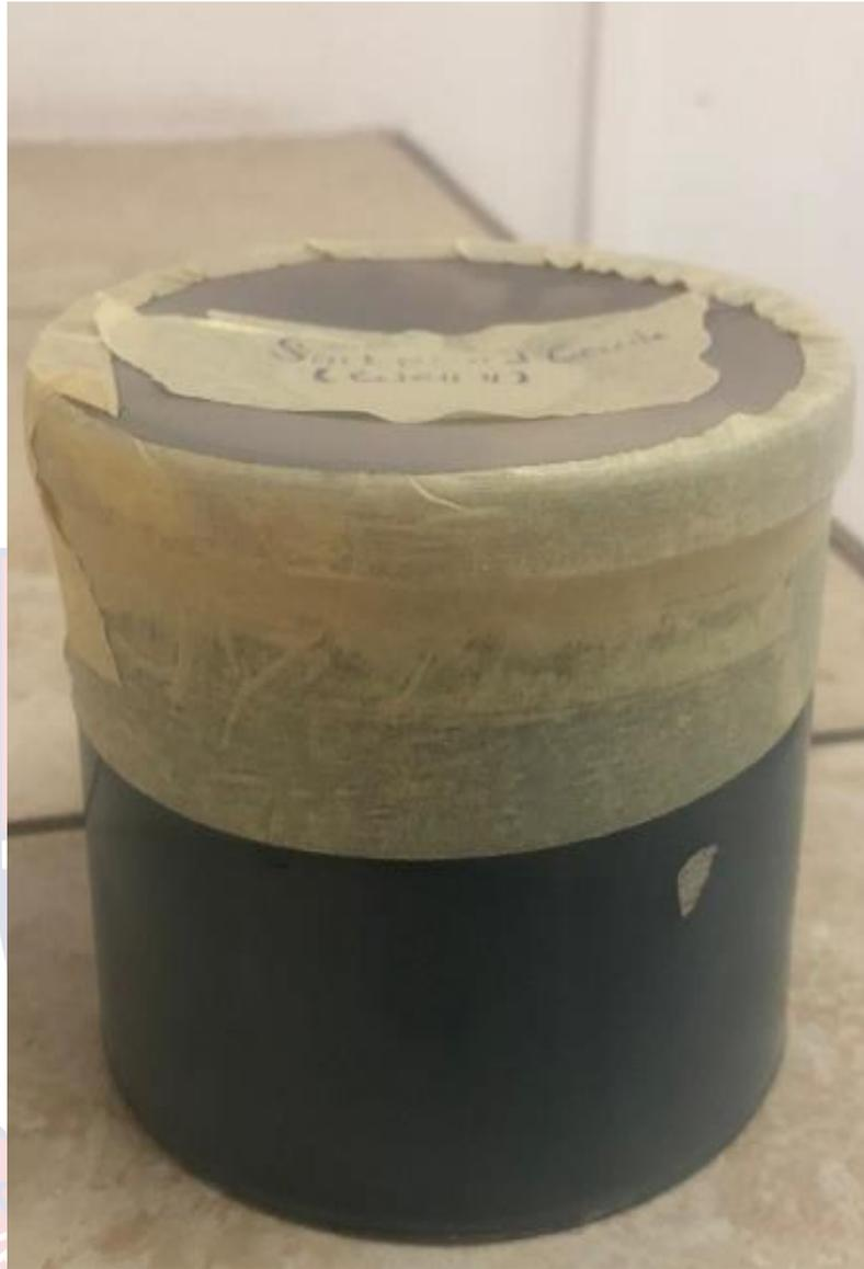
*Figure 16: Marinelli beaker filled with crude oil and sealed*
