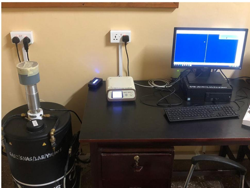
*Figure 18: DSPEC LF MCA -To- computer configuration*
