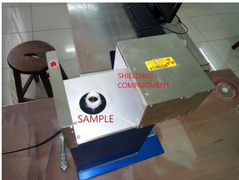
*Figure 14:* Sample holder in the shielding compartment of the AMPTEK EXP 1 X-123 XRF experimenter kit showing the sample-detector configuration
