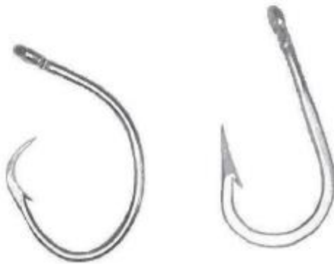
Plate 5. Circle hook (left) and J-hook (right) used in the pelagic longline fisheries (Source: Barkan, 2010).
