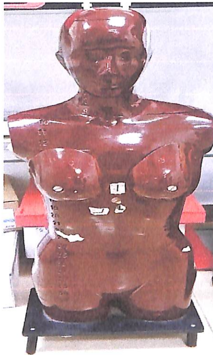
Figure 4: Picture of Rando (female) anthropomorphic phantom sectioned transversely for dosimetric studies.
