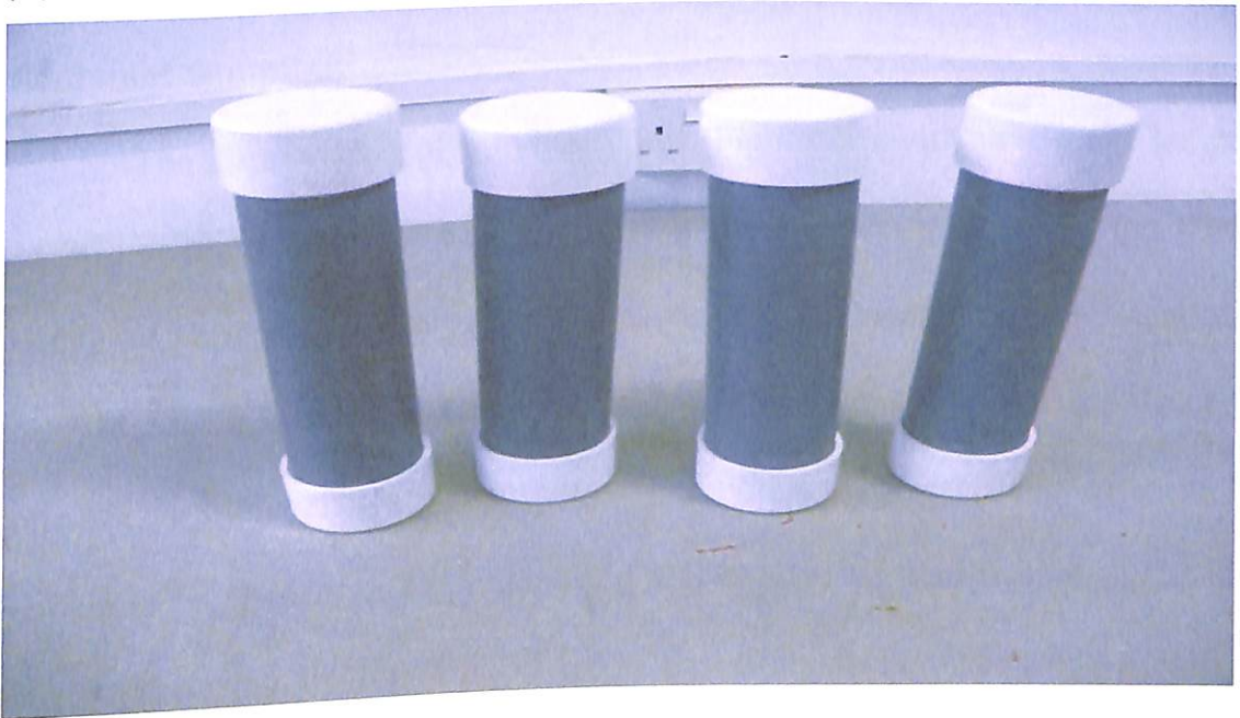
Figure 20: Improvised Corer (A & B) made of Polyethylene material with caps used in Sampling Sediment samples from the Pra River Basin in this Study Source: Author Data, 2013
