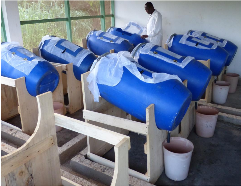
Figure 6. 4: Set up of larval density experiment (Arrangement of composting barrels in mosquito-netted composting shed)
