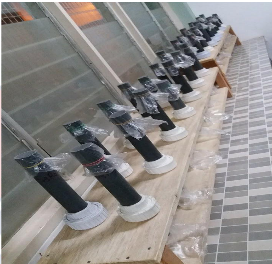
Figure 2: Soil Column Leaching Experimental Setup.
