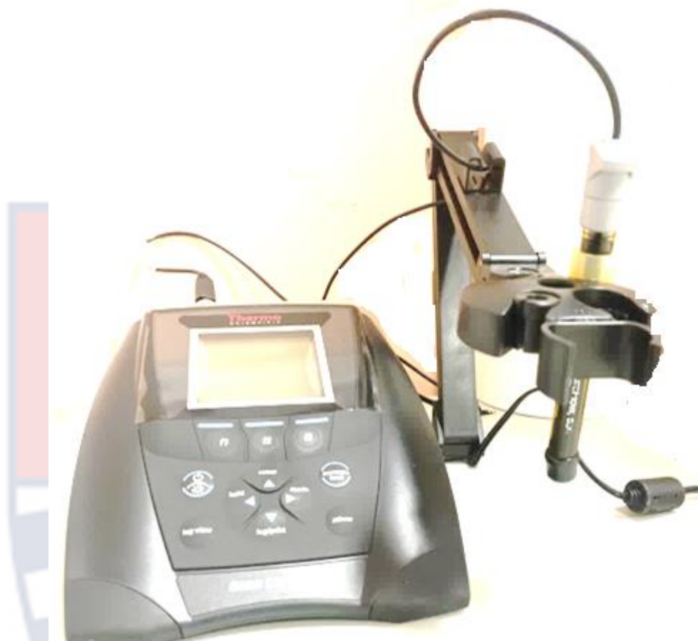
Figure 6: Electrometer with Fluoride Ion Selective Electrode
