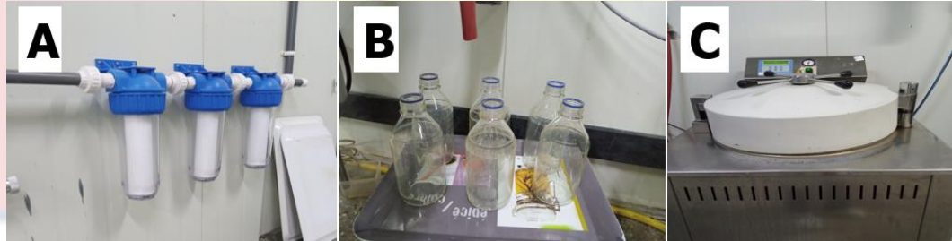
Figure 3: A - water filters, B - Glass bottles to be filled with filtered tap water, C - Autoclave
