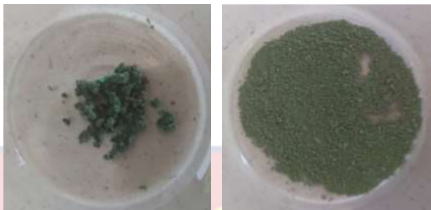
Figure 20: Images of synthesized Cu-5abdc (a) before activation (b) after activation
