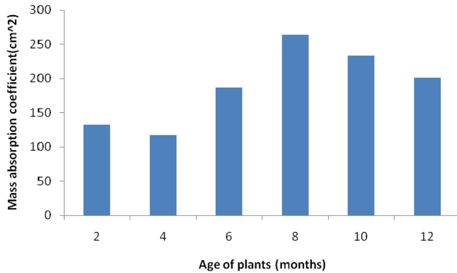
Figure 11. Relationship between averaged mass absorption coefficient versus age of plants (months) for all the three varieties
