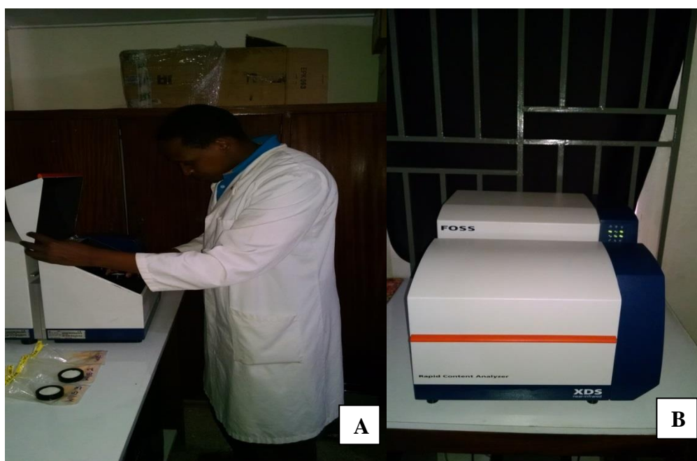
Figure 13: Biochemical analysis (A) and the NIRS Analyzer (B)
