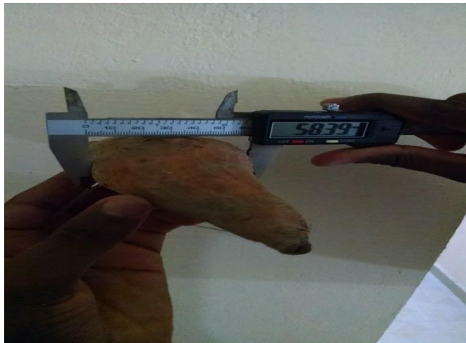
Figure 11: Shrinkage determination by use of a digital Vernier (accuracy 0.01)
