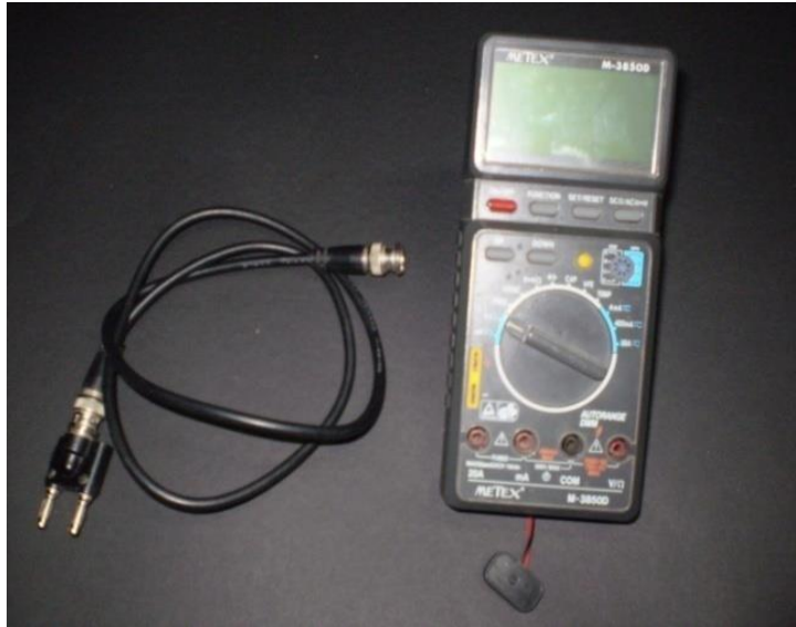
Plate 4: M-3850 D Metex instrument with its connecting cable
